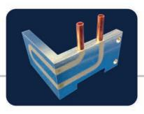
Pressed Tube below surface with high thermally conductive bonding epoxy back filled and fly cut. Great for opposite side cooling. A right angle transition is possible.
